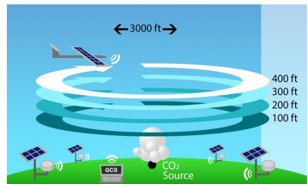
Figure 1 – Concept of a solar powered WSN and UAV gas sensing system.
