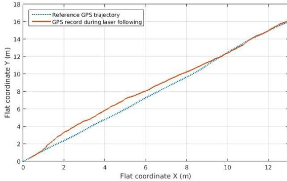
Fig. 7. Result of footprint tracking evaluate with RTK GPS
