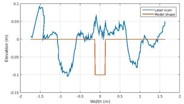
Fig. 3. Example of laser scan with two tire footprints and the associate template use in correlation
