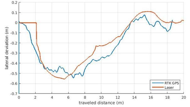
Fig. 8. Lateral deviation compare between lidar detection algorithm and RTK GPS
