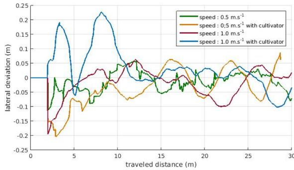
Fig. 10. Lateral deviation at different speed and with or without cultivator
