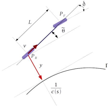
Fig. 2. Simple bicycle model applies to path tracking
