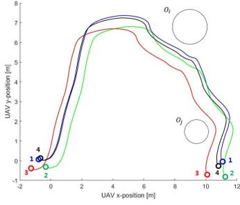
Fig. 5. Trajectory of UAVs projected on the XY planes during the task.
