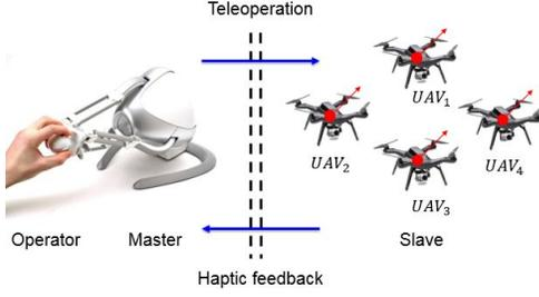
Fig. 1. Concept of a multi-UAV System: haptic teleoperation of multiple UAVs
