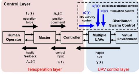
Fig. 2. Two control layers while using teleoperation
